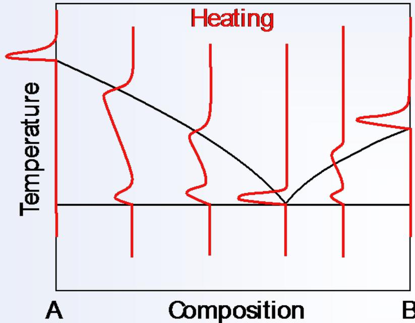
DTA response superimposed on phase diagram of a simple eutectic system with no solid solubilities (equilibrium heating and cooling)
