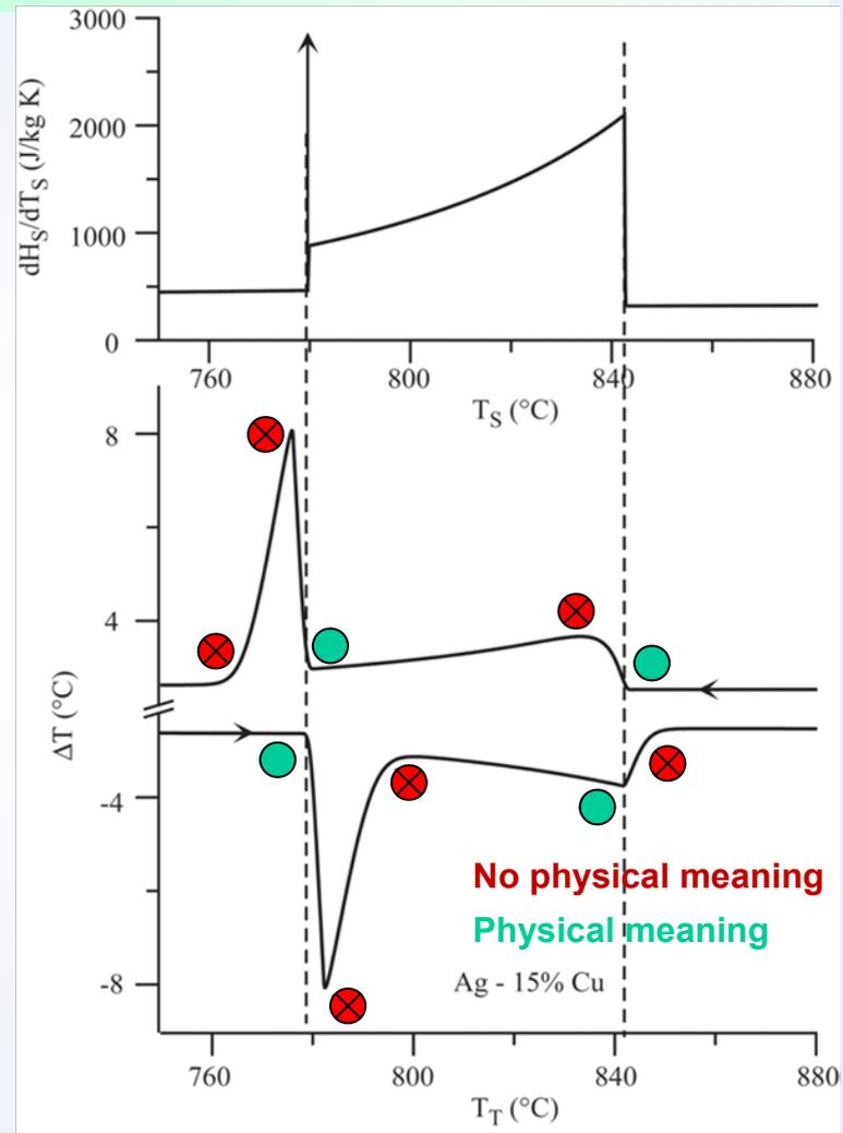
Unless  $dH_S/dT_S$  shows a delta function, there is **NO** physical basis for linear extrapolation of the DTA curve!
