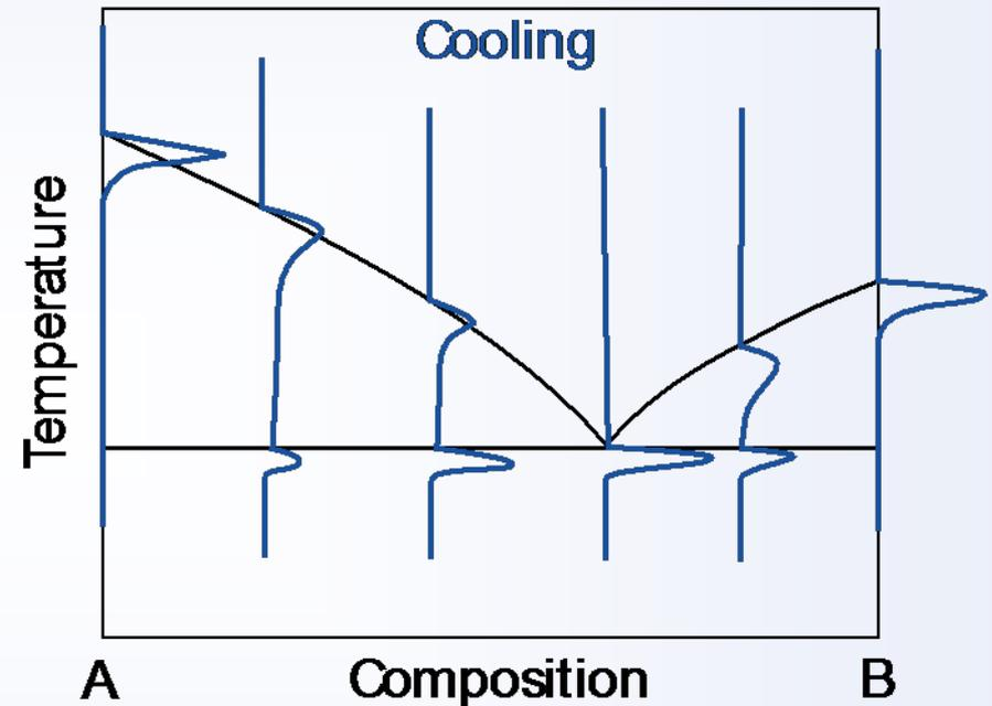
**Note the different signal shapes on heating and cooling!**
