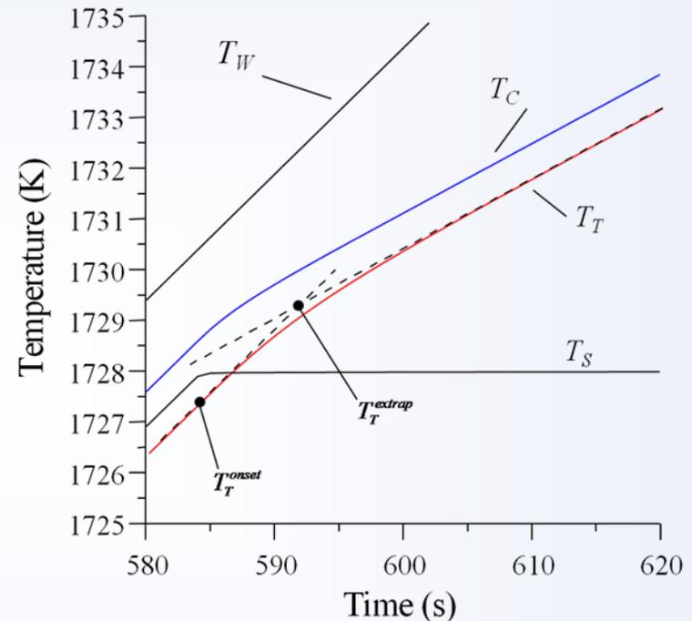
As result of thermal conductivity, the temperature of the sample thermocouples lags behind the actual sample temperature
